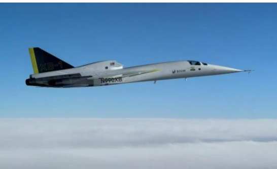
Above: Boom Supersonic’s jet has three engines, one on top and two on the sides of the fuselage. Its wings are swept back to make it stable at high speeds.
